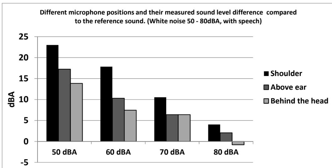
Figure 3: Background noise measurements using white noise with speech contribution from the microphone carrier compared to reference measurement
