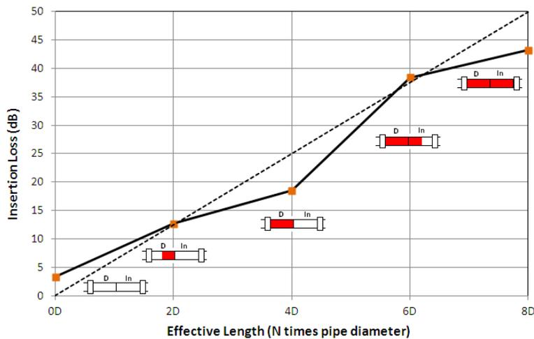
Figure 8: Sound insertion loss (dB) function of effective length of the pipe array (0D to 8D). The drawings illustrate the corresponding pipe array configuration where red colour indicates the active area of the array. Discharge pipe is designated with a “D”; inlet pipe is labelled “In”
