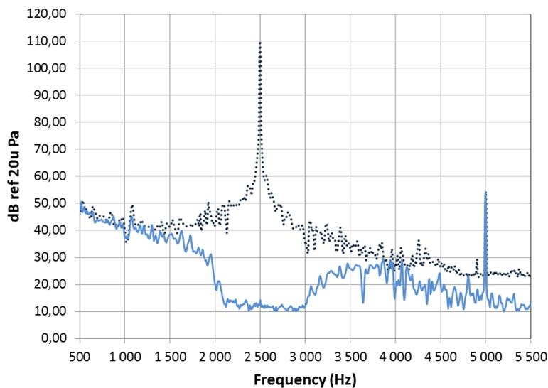
Figure 6: Measured sound pressure level (dB) of combined effect of both discharge and inlet pipe arrays in series. Effective length 8-diameter (8D). Tonal noise
