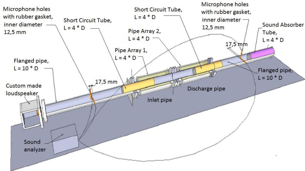
Figure 3: Measurement set up (illustration by [6])
