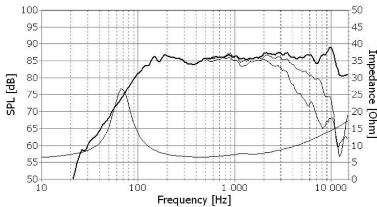
Figure 4: Loudspeaker frequency response (Seas H1304-08A12RC) [7]
