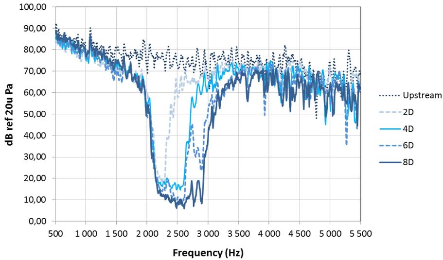
Figure 7: Measured sound pressure level (dB) with variable effective length of the pipe array (2D to 8D)
