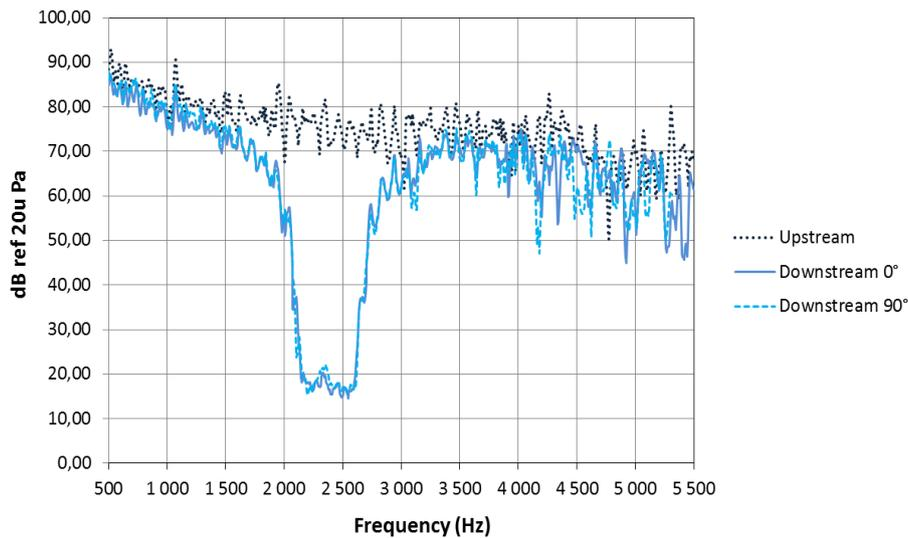
Figure 10: Comparison of sound pressure level (dB) between spool configurations in-series (solid line) and separated with a 90° bend (dotted). Effective length 4D
