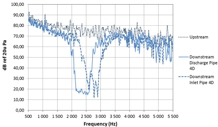
Figure 5: Measured sound pressure level (dB) downstream of discharge (solid line) and inlet (dotted line) pipe arrays. 4D effective length. Random noise
