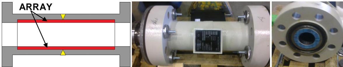
Figure 2: Left, sketch of pipe spool with pipe array (illustration by [5]); Middle, 4D pipe-spool; Right, detail of pipe spool with pipe array inside
