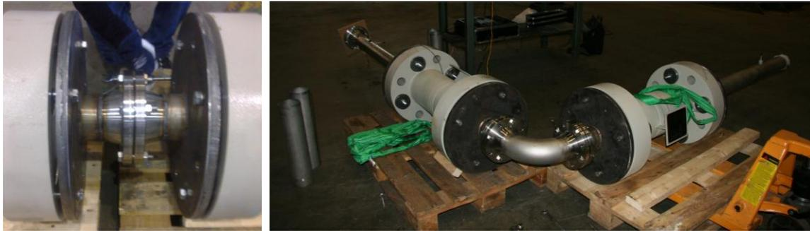
Figure 9: left, in series configuration; right, pipe arrays separated by a 90° bend.
