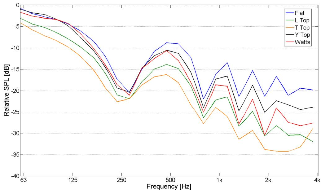
Figure 5: Insertion loss 20 m behind the different types of barrier as a function of frequency.
