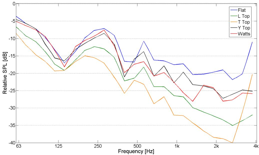
Figure 4: Insertion loss 10 m behind the different types of barrier as a function of frequency. For this case, the barrier is absorbing and the ground is rigid.
