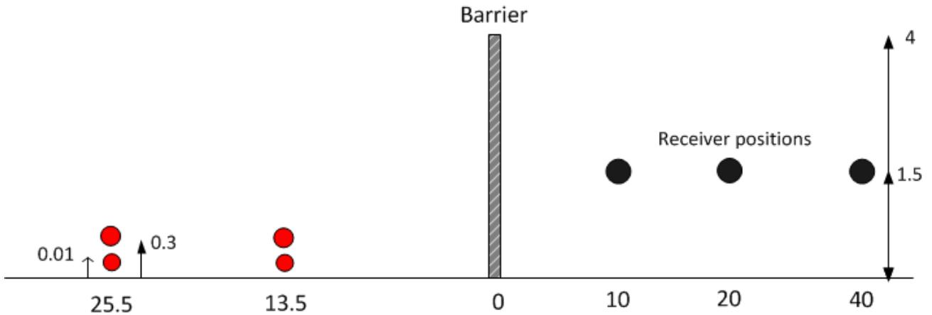
Figure 2: Cross section describing the simulated situation. Each driving direction with two lanes is simulated by two sources (red dots) and the receivers are represented by black dots. Distances and heights are in metres; the figure is not to scale
