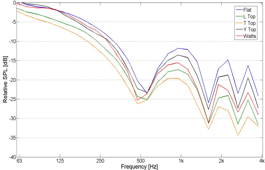
Figure 6: Insertion loss 40 m behind the different types of barrier as a function of frequency.
