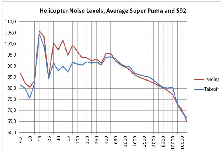
Figure 1: Practical Offshore Helicopter Noise Spectrum, 40 m Distance
