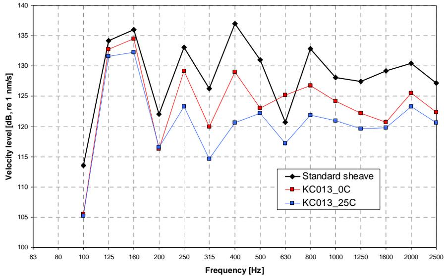
Figure 3: The effect of temperature on the behaviour of a single epoxy damper ELASTE\_KC013. The optimal operational temperature of that epoxy system is at 25 °C.
