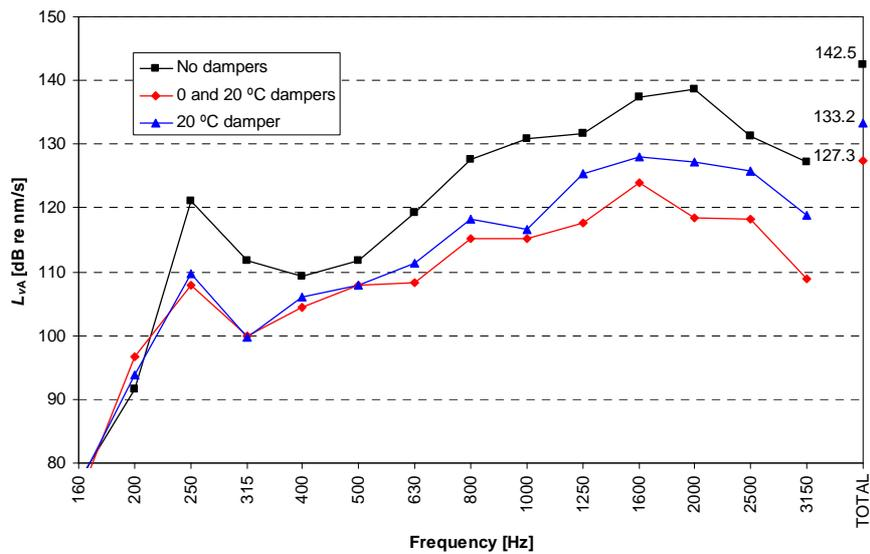
Figure 5: A-weighted velocity level in point 2 for a unit force excitation in the driving point.
