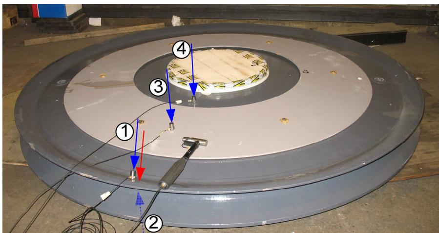
Figure 4: Measuring positions. Excitation position (the driving point) is shown with the red arrow and response accelerometers 1 to 4 with blue arrows. Response point 2 is on the underside of sheave. The light grey area is the constraint layer damper.
