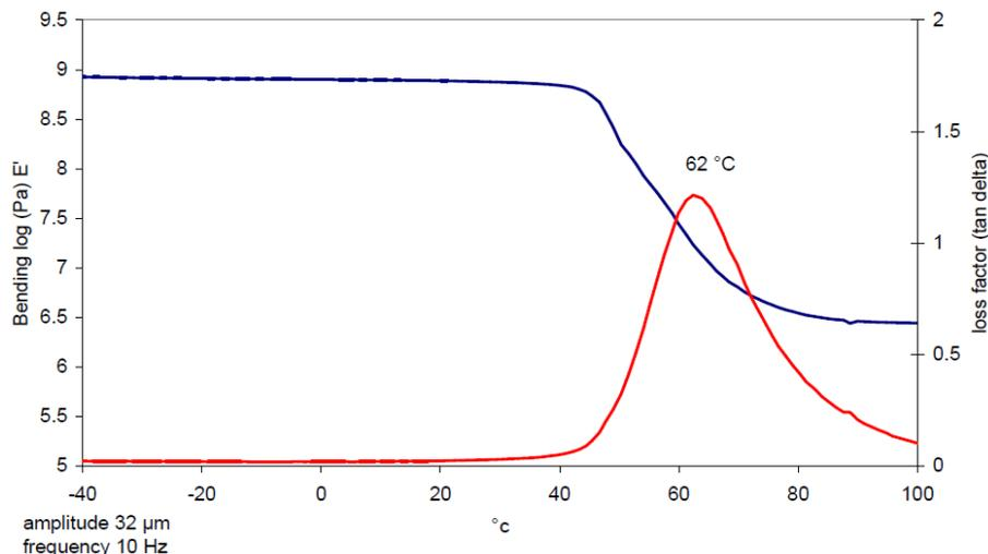
Figure 1: A typical DMTA measurement curve of a high damping epoxy system displaying a change in storage modulus (black curve) and change in loss factor (red curve). The limits of  $T_g$  region are 40 °C 90 °C and the value of peak loss factor of 1.25 is at 62 °C. The region exceeding loss factor of 1.0 is located in between 55 °C 70 °C when frequency is 10 Hz and amplitude is 32 μm.
