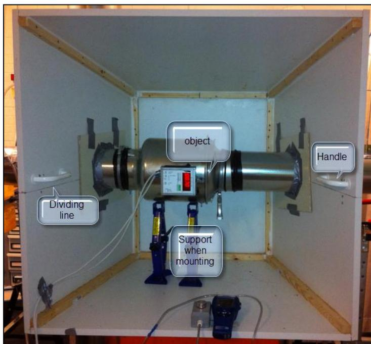
Figure 1 Ventilation unit mounted in sound reflector box. Opening surface area is 1 m<sup>2</sup>.
