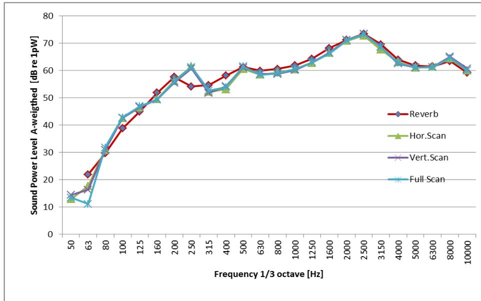
Figure 4 Test Sound source measured in Reverberation Room, and in Reflector box using Horizontal, Vertical and Full scan.
