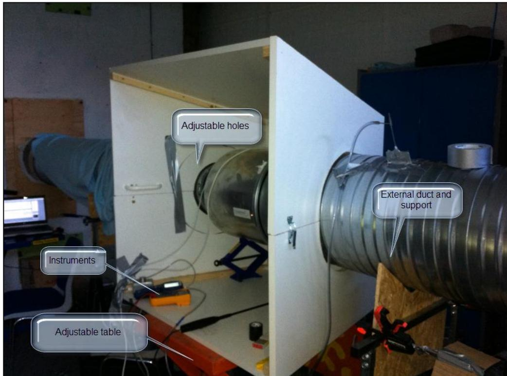
Figure 3 Example of a setup for measuring very sound power levels from a ventilation unit in a laboratory with other background noise sources. Pressure loss is measured on the suction side of the ventilation unit.
