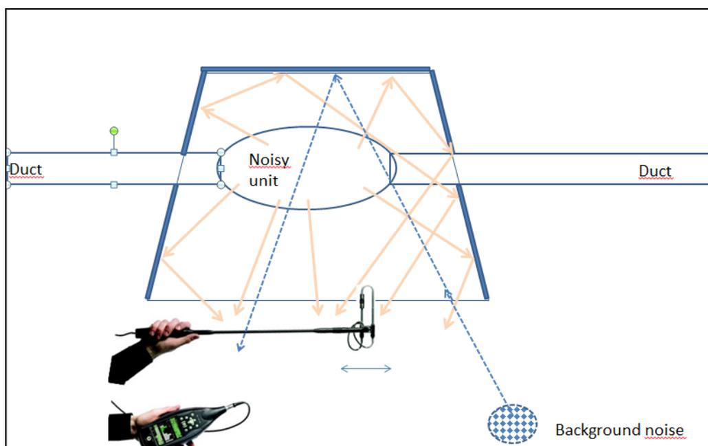
Figure 2 Principle for reflection of emitted noise and background noise. Intensity probe is moved on the opening surface in a systematical pattern (scanning).
