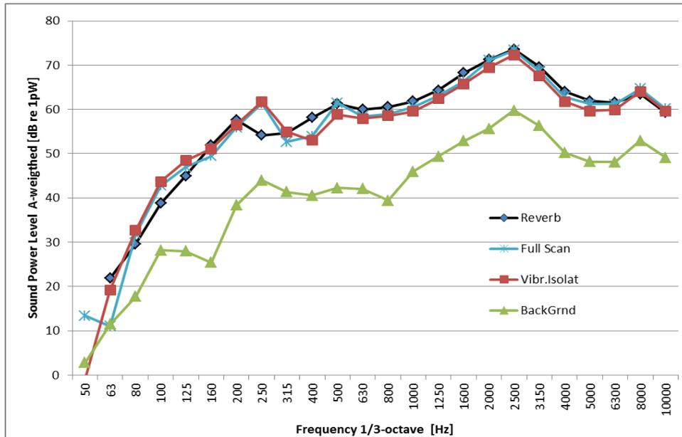
**Figure 5** Survey test of vibration isolation of loudspeakers and of background noise source outside the reflector box.
