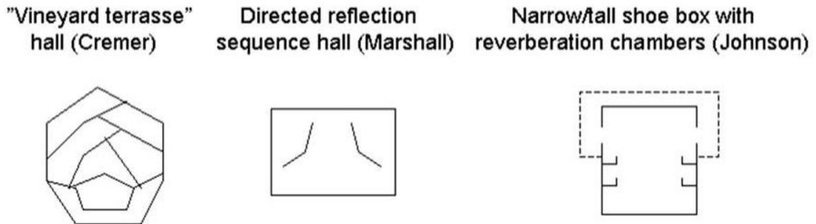
Figure 1: Sketches of three different concert hall shapes capable of achieving both high clarity and high reverberance
