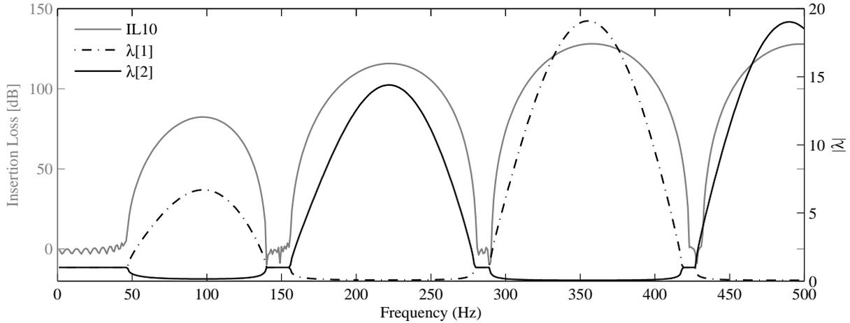
Figure 5: Insertion Loss (IL) at 10 cell periodic beam structure (FEM) and Bloch parameter ( $\lambda = \exp(-iK_B)$ ) (Floquet theory) within 0 to 500 Hz frequency range
