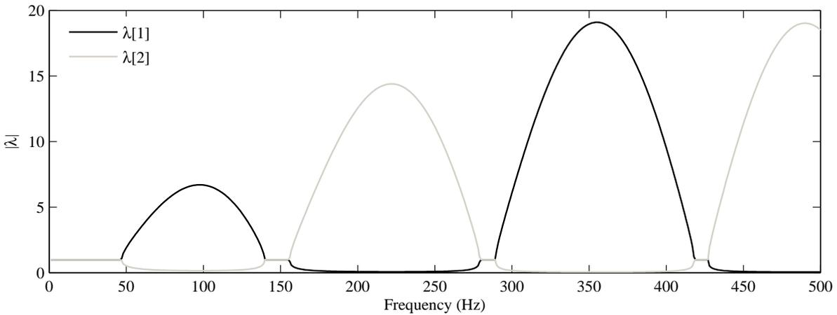
Figure 4: Bloch parameter ( $\lambda = \exp(-iK_B)$ ) for infinite beam structure (Floquet approach)
