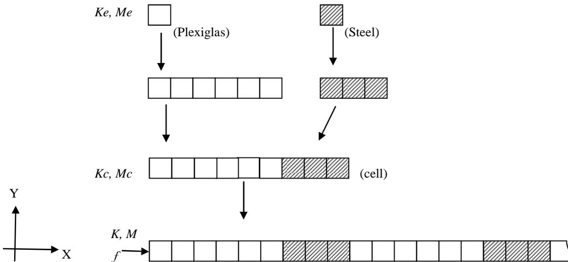
Figure 1: Formation of semi-infinite beam structure using FEM approach ( $K_e, M_e$  = Stiffness and Mass element matrices,  $K_c, M_c$  = Stiffness and Mass cell matrices,  $K, M$  = Stiffness and Mass system matrices)
