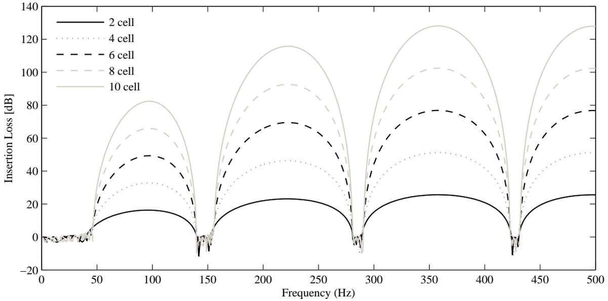
Figure 3: Insertion loss (IL) for wave propagation in the periodic semi-infinite bar structure within the 0 to 500 Hz frequency range
