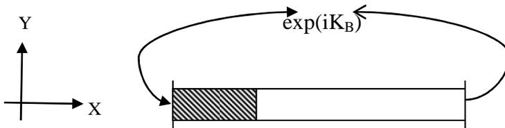
Figure 2: Formation of beam structure using Floquet approach
