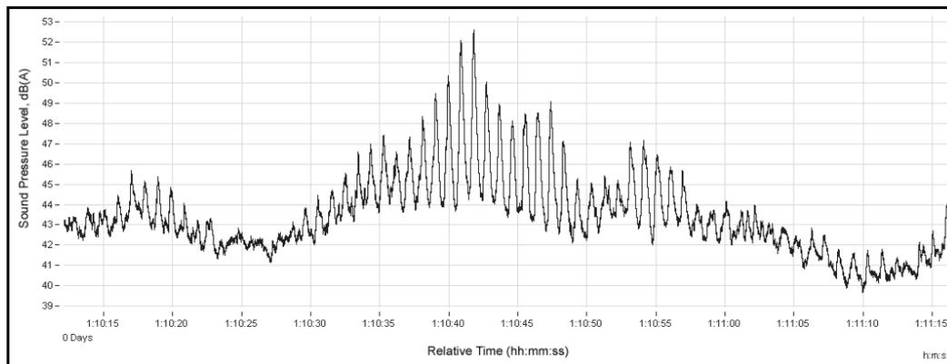
Figure 1. Amplitude modulation of wind turbine noise recorded in far field location. The time frame of the picture is 60 seconds.
