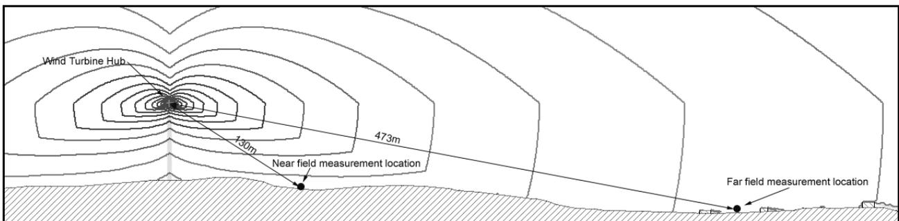
Figure 2. Sound level contours with a 3 dB level class from a vertical grid calculation. Upper level and upwind directivities are only assumed.
