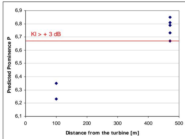
Figure 3. Modulation impulsivity in two measurement points according to the Nordtest method
