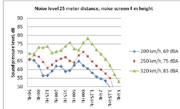
Figure 8. Noise from high speed train with different speed at 25 meter distance, 4 m noise screen.
