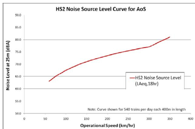
Figure 3. From British studies of high speed lines. Day time average noise level ( $L_{eq,06-18}$ ) at 25 meters. [4]
