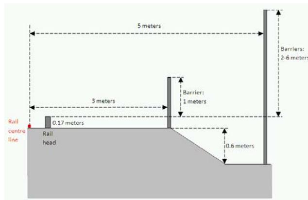
Figure 5. Embankment and position of barriers
