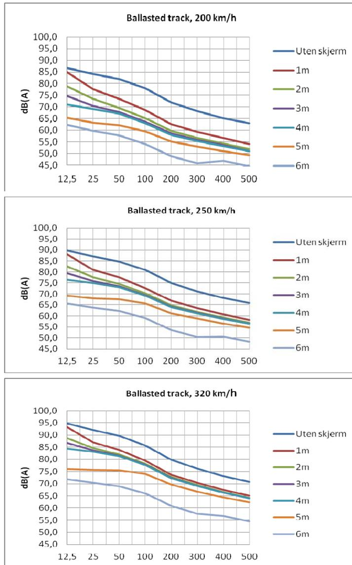
Figure 6. Calculated maximum free field noise levels for different speed, distances and screening
