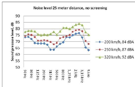
Figure 7. Noise from high speed train with different speed at 25 meter distance.
