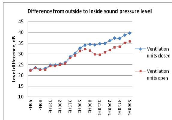
Figure 9. Noise reduction in wooden houses: arithmetic mean value from 83 measurements.
