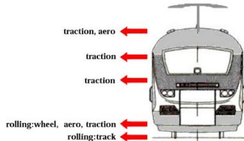
Figure 4. Vertical distribution of railway noise sources [6].
